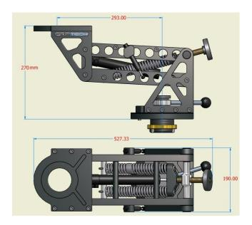
QUICK ACTION SWIVEL FEATURE ENABLES YOU TO ROTATE THE ARM 360 DEGREES AND LOCK.
