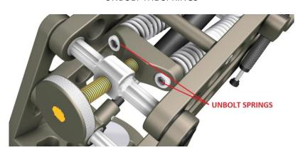
AFTER CHOOSING AND INSTALLING SUITABLE SPRINGS, ENSURE THAT THE SPRING BRACKET IS ORIENTATED CORRECTLY BEFORE PROCEEDING.
