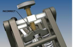
MOUNT THE CAMERA PACKAGE AND WIND THE LEVEL ADJUSTER KNOB IN OR OUT TO RAISE OR LOWER THE ARM TO A LEVEL POSITION.
