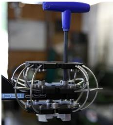
Mounting the camera batteries on the top plate of the WRI has proved to have a stabilising effect on the image as well as a convenient place to put cumbersome batteries. Weight of up to 4kg can be mounted on this plate to further soften the ride.
