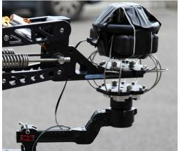
With the gimbal and camera attached, note what angle the arm is. The arm should lie just above horizontal for best results. If it lies below the horizontal, adjust the springs with an Allen key by screwing clockwise. Make sure that both springs, when adjusting the tension are done evenly. For example one spring has approximately the same amount of turns as the other.
