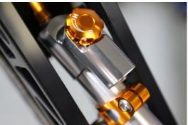
With the arm now lying level or just above the horizontal (with the payload attached), push down on the front of the arm and note the movement of the arm. The arm should come to rest with 3 or 4 movements. If the arm continues to bounce up and down, turn the adjustment knob on the damper towards the H (Hard). Turn in the opposite direction if the arm is too rigid.
