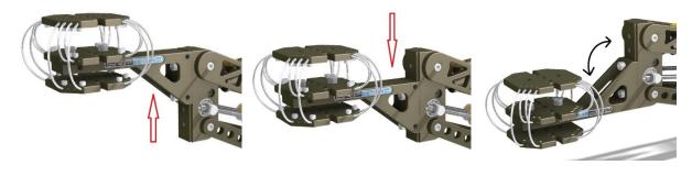
The WRI (Wire Rope Isolator) is easily attached to the nose bracket of the VVI using 2 x 3/8 UNC cap screws. The WRI is mostly mounted with the camera and Gimbal "hanging" from the bottom plate although a camera can be attached to the top plate without a Gimbal. The WRI can interface with the Movi (Toad in the Hole) and the Ronin (with the Cinemilled Ronin plate).
